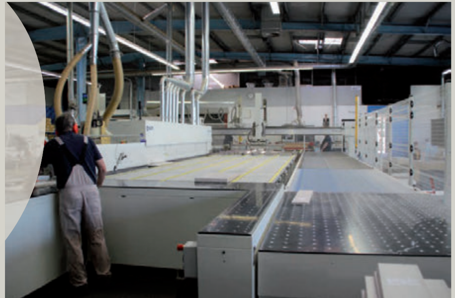
The 'stefani cell E' edgebanding cell in action at the plant based in Lauffen am Neckar.
