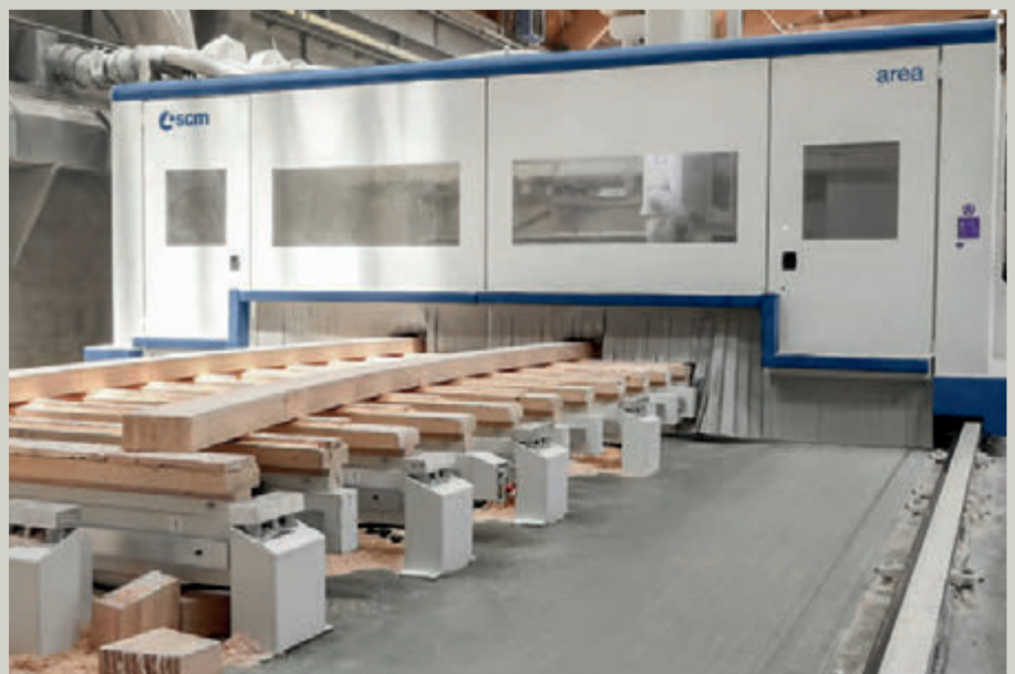
The "area" cnc machining centre in action at the Jagram-Pro plant. Above, a detail of the machine.
