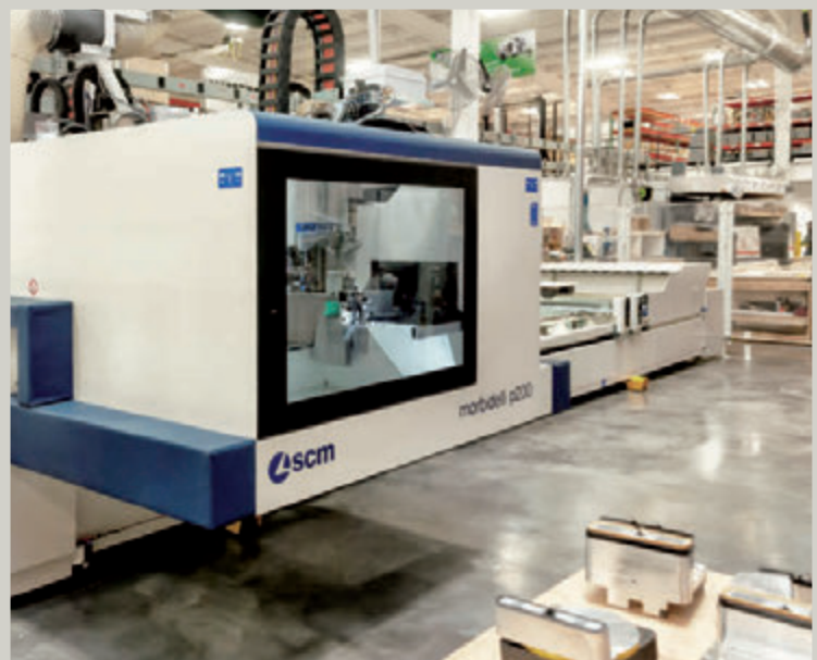
The "morbidelli p200" cnc machining centre with the exclusive HE-POD suction cup system.
