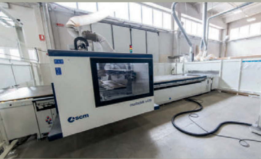
Two images of the "morbidelli x400" cnc machining centre.
