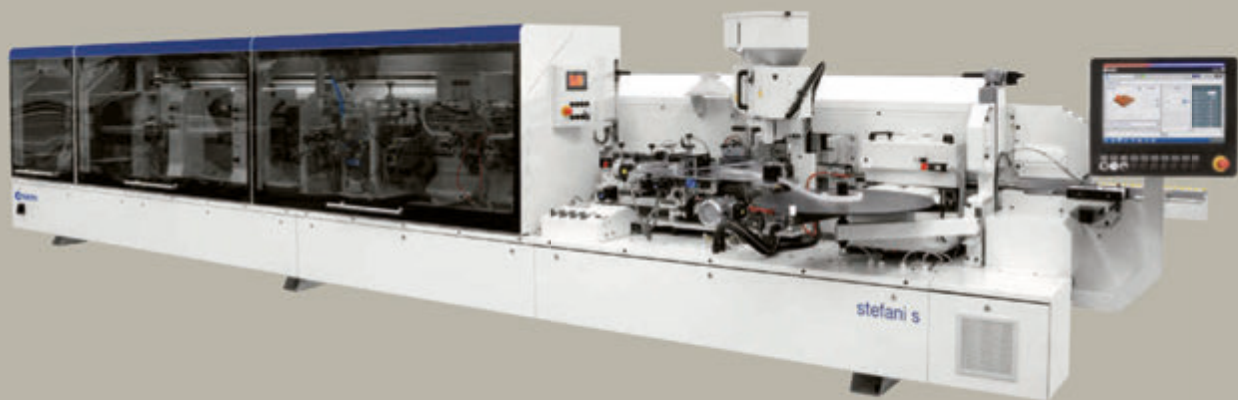
General picture of the 'stefani s' edgebanding machine chosen by HanseYachts. Above is a machining detail and some of the beautiful furniture made by the German manufacturer.
