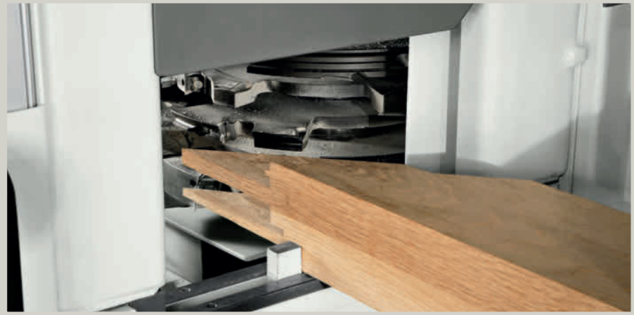
Tenoning operations with the "windor nt 1" machining centre.
