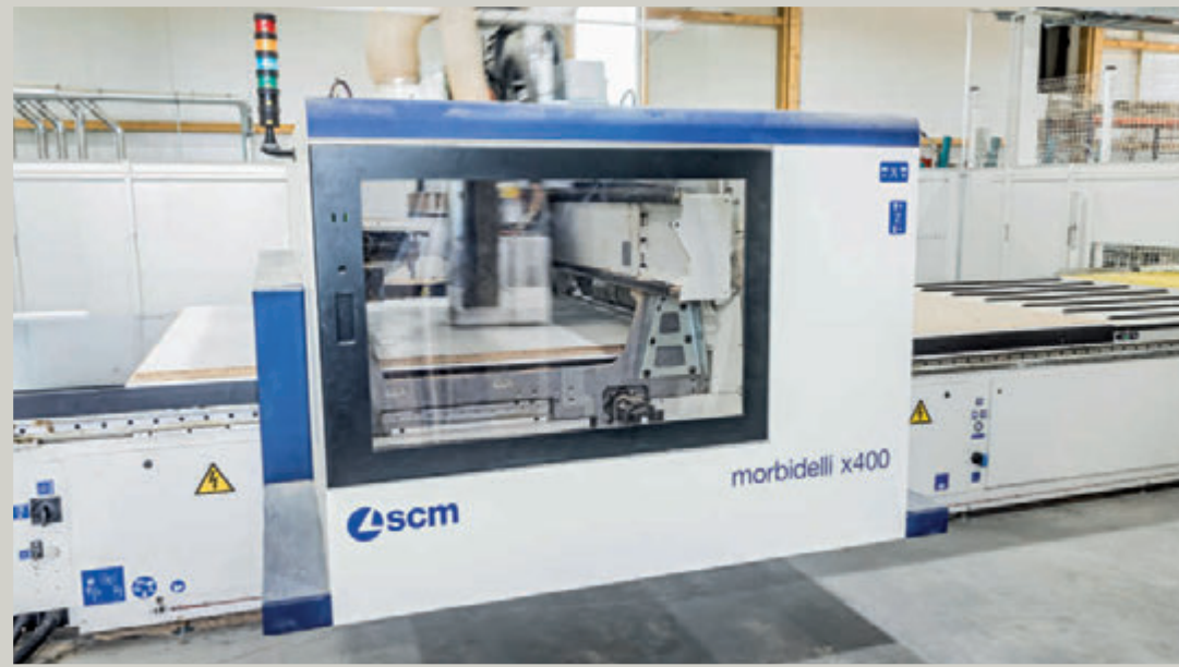
The 'morbidelli x400' cnc machining centre is integrated in a 3-axis automatic storage, 'flexstore el' (pictured above) that optimises the panels handling.
