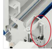
Pressure beam Maintenance-free thanks to the mechanical solution that involves the movement of the pressure beam on prismatic guides
